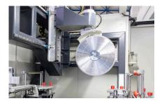
550 mm diameter saw that can cut at any angle between 0° and 180° thanks to its 4-axis movement capability, the saw allows cutting and end-milling operations of profiles up to 320 mm wide.
